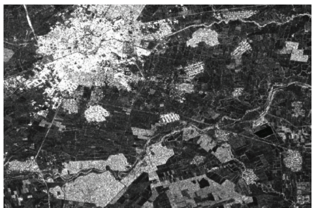
Figure 1b. Sentinel-1A image, VH polarisation, 10 m spatial resolution (© Copernicus Sentinel data 2017)
